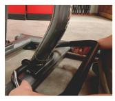
1) Place Sit up bar (L) on spine bolts with the rounded side up.
