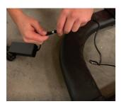
4) Attach end of DC Power Cable (M) from bottom of Spine into AC Power Brick (P) and plug into wall.
