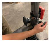
3) Loosen knobs to adjust to appropriate height. Tighten knobs fully before use.
