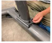
3) Screw the 4 Fasteners (M10 Nylock Nuts (E) & M10 Washers(D)) into place. Be sure not to tighten fasteners all the way.
