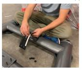
1) Remove 3M Tape from Rubber Gasket (H) and place on the rear spine bolts.
